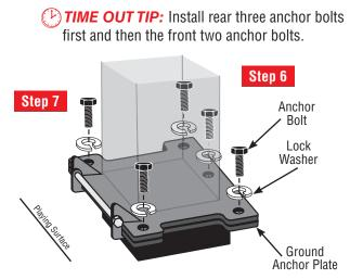
**Step 9:** Snug tighten the five anchor bolts, then check goal assembly with a level and inspect visually to determine if it is parallel and plumb to the playing surface.
