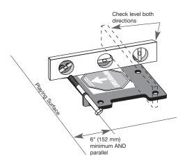
**Step 6:** Position 4" ground anchor (Item G2440) in center of hole with hinge side toward and parallel with playing surface. Using a level, ensure the anchor is level front-to-back and left-to-right. All edges of the ground anchor must be 6" (15.2 cm) away from all sides of hole and the top of the ground anchor within a range of 1"- 3" (25-75 mm) above the level of the playing surface.
